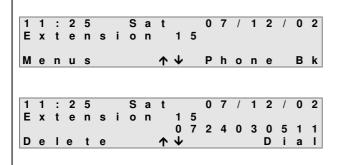
With the telephone idle, to make an external call simply dial the line access digit or the line access group, followed by the external number from the keypad.
